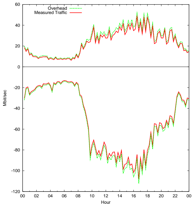
Figure 11: Traffic and correspondig tunneling overhead in a one daylong report (negative values express incoming traffic).
