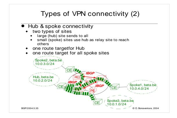
In this example, Hub, beta.be is used as a transit router for all packets exchanged between any sites of the VPN.
