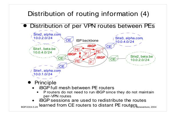
If the ISP network is large, the iBGP full-mesh can be replaced by the classical iBGP scaling techniques that are Route Reflectors and Confederations. In the case of Route Reflectors, a PE would typically be client of two Route Reflectors and the Route Reflectors would be fully meshed. The iBGP sessions used for normal Internet routing and for VPNs can be the same or different. In some ISPs, a different iBGP distribution is used for the VPNs.
