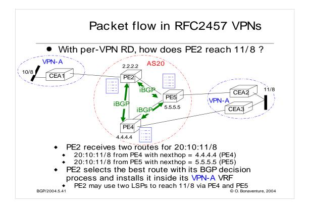
In this example, we assume that the route target used by PE5 is 20:10 (20 because the AS number of the ISP and 10 is the number allocated by the ISP for VPN-A, assuming per-VPN route targets)
