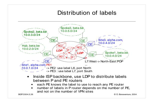
LDP is the common way to distribute the labels to reach the PE routers in the backbone. However, the PE-PE MPLS LSPs could also be traffic engineered tunnels established with RSVP-TE.
