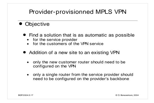
The provider-provisionned MPLS VPNs are defined in RFC2547 BGP/MPLS VPNs. E. Rosen, Y. Rekhter. March 1999.
