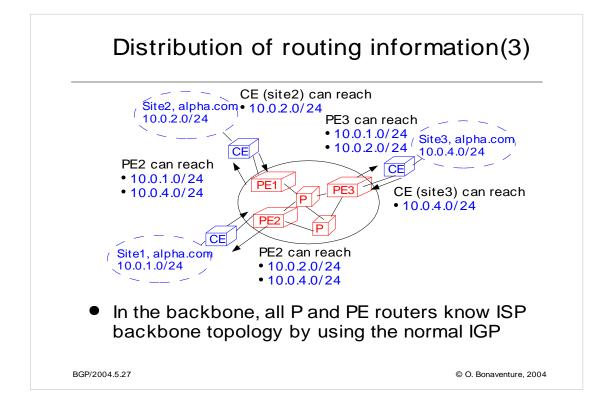
In this example, the routes between the CE and the PE routers can be exchanged by using any of the protocols discussed in the previous slide.
