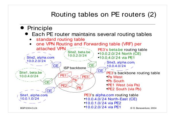
The VRF contains all the routes belonging to a given VPN. This VRF is used to forward the packets that are received inside the corresponding VPN. For example, when considering PE3, it will use the beta.be VRF to forward a packet received on its North interface while it will use the alpha.com VRF to forward a packet received on its North-East interface.
