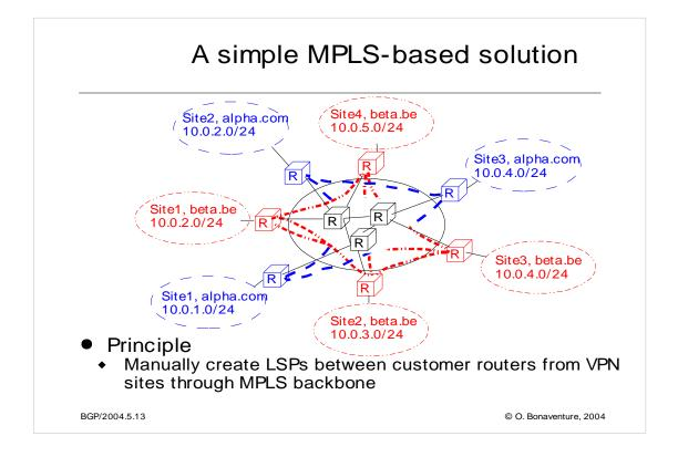
This simple MPLS-based solution is similar in principle to the solution used to support VPN with technologies based on the label switching paradigm like
