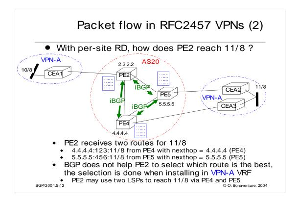
In this example, 123 and 456 are locally unique numbers managed by PE4 and PE5.
