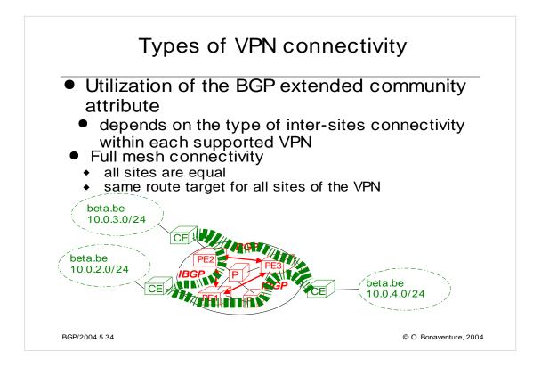
In the figure above, the dotted lines show the packet flows between the CE routers of the beta.be  $\ensuremath{\mathsf{VPN}}$
