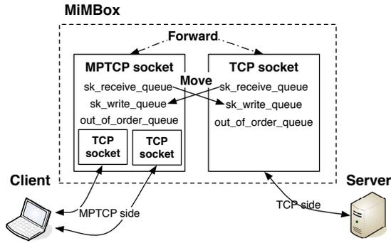
Figure 2: MiMBox maintains fully-functional sockets and forwards in-order segments from one side to the other.
