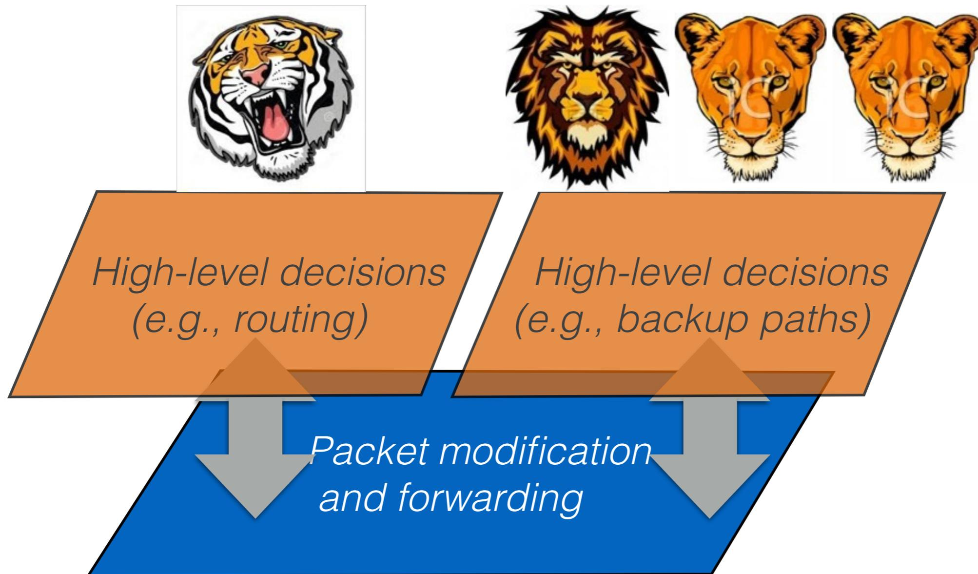
Operators can and *do run coexisting control-planes*, that work independently from each other
