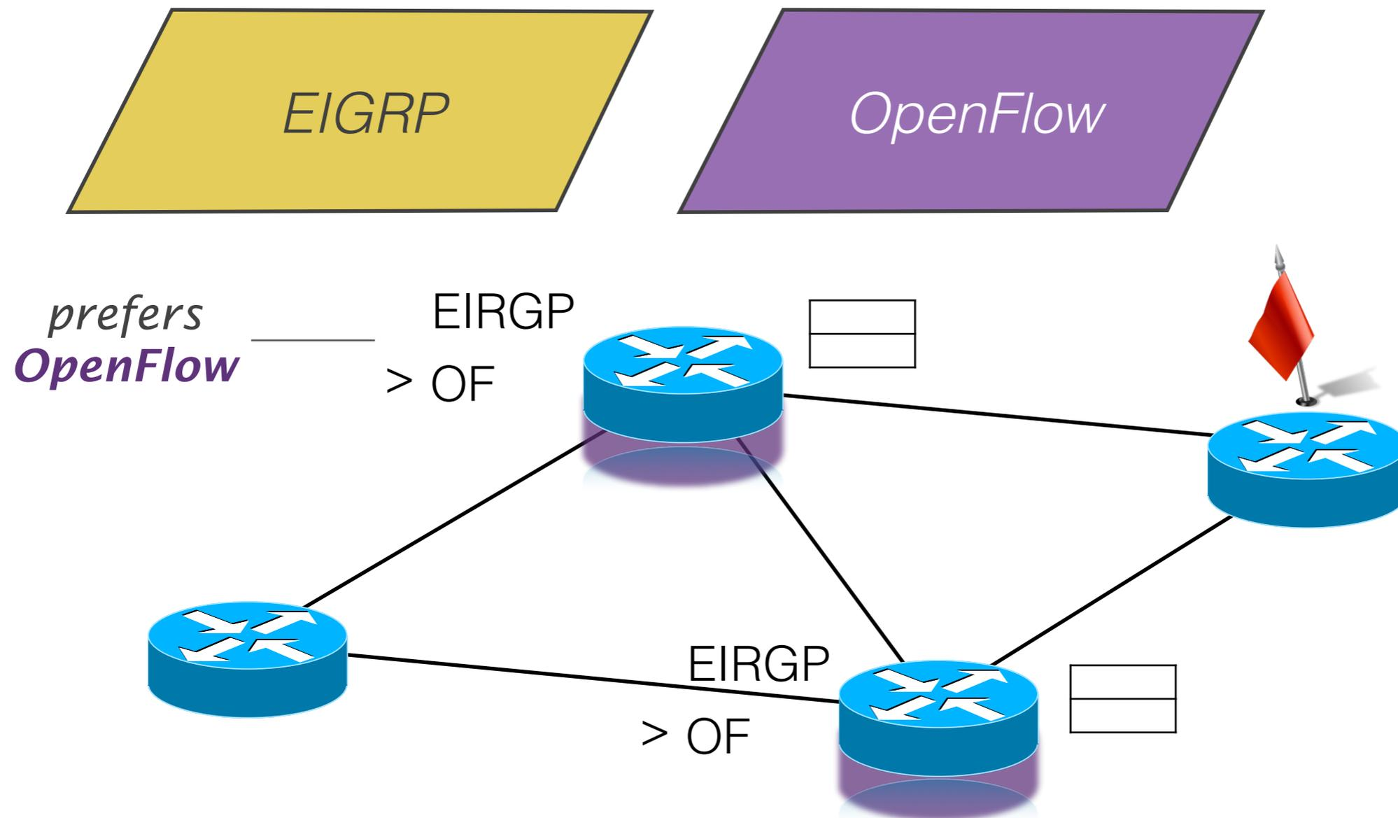
Being preemptive, OpenFlow directly writes to the FIBs of the routers
