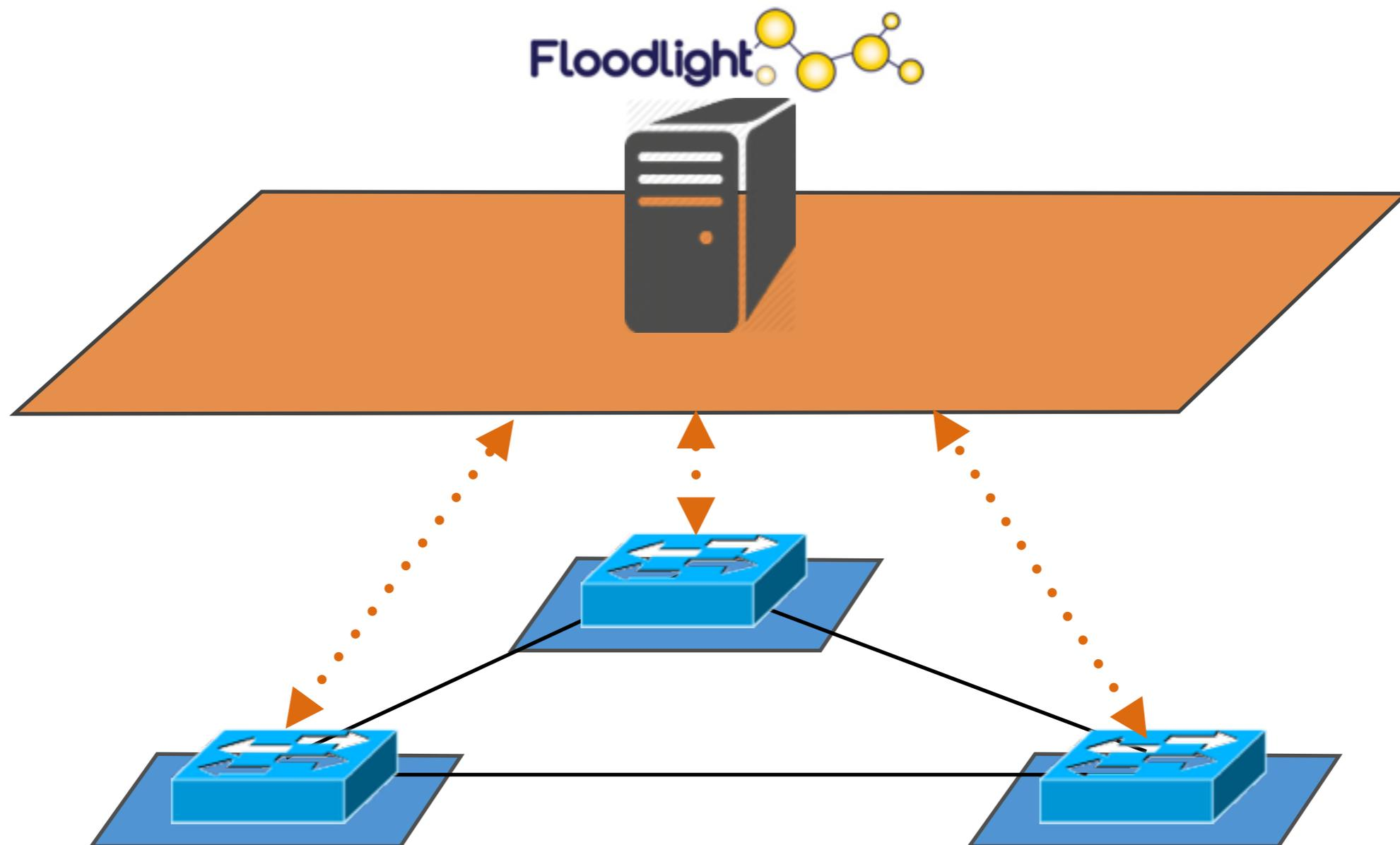
SDN is based on control-plane centralization
