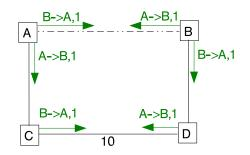
Fig. 5: The first wave of reply HELLO PDUs when link  $A \rightarrow B$  fails gracefully
