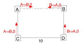
Fig. 8: The first wave of HELLO PDUs when link  $A \rightarrow B$  comes up in the simple network
