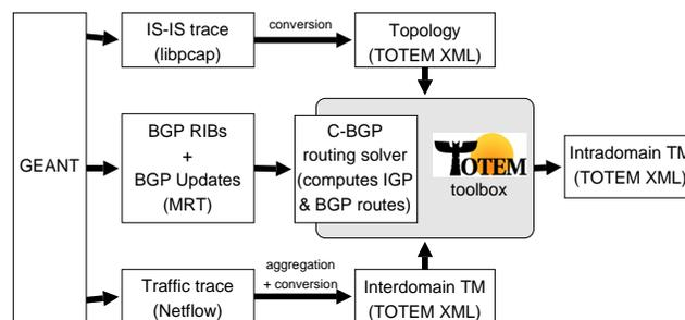
**Figure 3: Architecture of the TM generation setup.**
