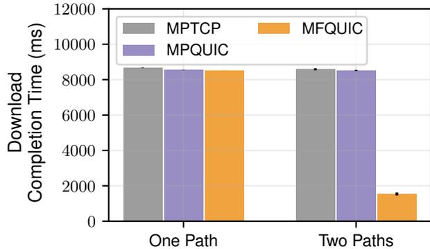
Fig. 4. When the secondary path has a very high asymmetry, MFQUIC benefits from it while both MPTCP and MPQUIC cannot. Error bars show standard deviation over 15 runs.
