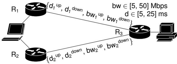
Fig. 3. Network topology used for asymmetric experiments.
