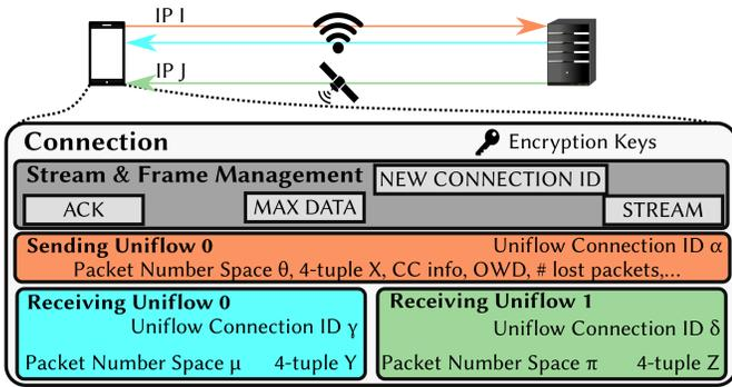
Fig. 1. State of a Multiflow QUIC connection from the client's perspective. The client has IP I when using the upper network path, and IP J when using the lower one.
