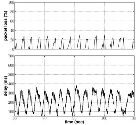
**Fig. 7.** Downlink – delay and packet loss (18:00 test)
