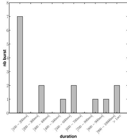
**Fig. 6.** Downlink – loss bursts duration distribution (12:00 test)
