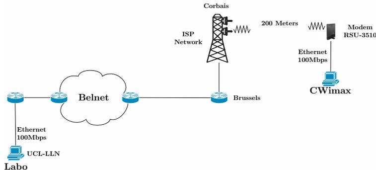
**Fig. 1.** WiMAX testbed for TCP measurements
