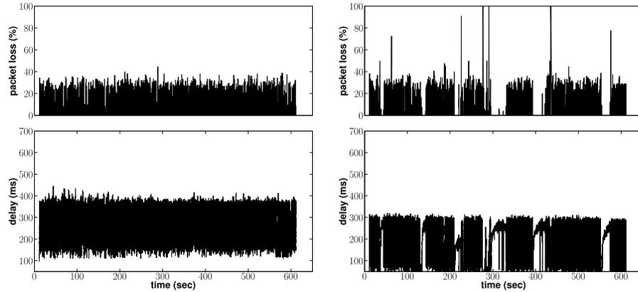
**Fig. 4.** Downlink – delay and packet loss (22:00 test) **Fig. 5.** Downlink – delay and packet loss (12:00 test)
