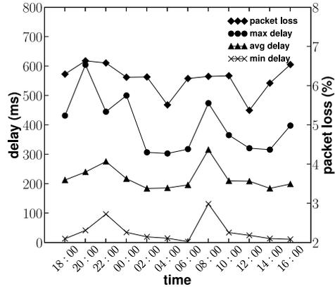
**Fig. 2.** Downlink - min, max, avg RTT values and deviation (whole day) **Fig. 3.** Downlink - delay and packet loss (whole day)
